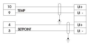
Screened Cable should be used to reduce EMI.
